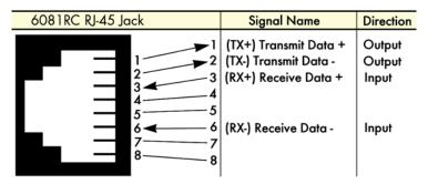
Figure 8. Ethernet RJ-45 pin and signal definitions for Model 6081RC
